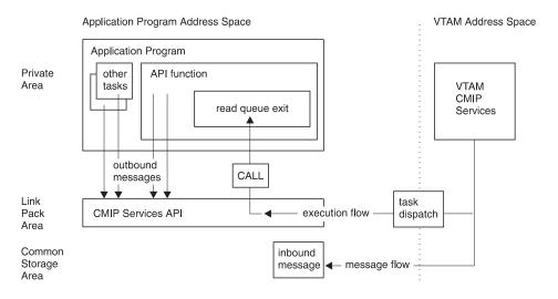
Figure 1. Using CMIP services with the common storage area interface
